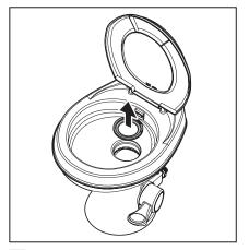
19 Removing the Flush Ball Seal
