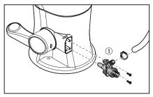
17 Removing the Water Valve Assembly(1) Water Inlet Valve Assembly
