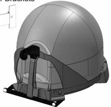
Allows hanging of antenna unit on vehicle window or included hanger bracket.
