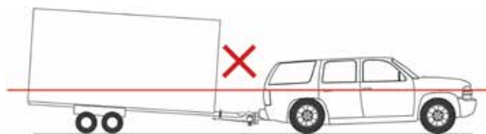
BAD: Far too much weight on back of tow vehicle Trailer is severely off-level 1. Check the Load 2. Check Installation 3. Tighten Tension Nuts
