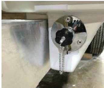
Rear Water Inlet located to the right of the rear bumper
